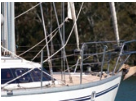
750mm stanchions fastened with 4 x 8mm bolts
