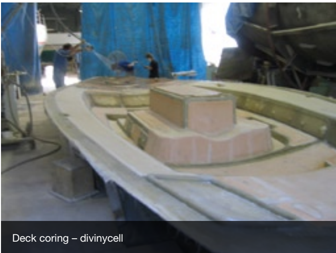
Solid coremat / GRP layers where deck fittings are bolted through
